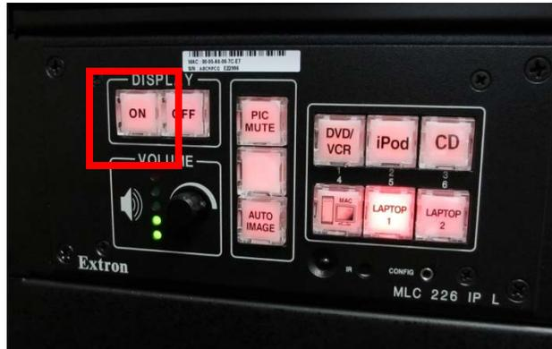
Selecting the On button on the Control Panel
